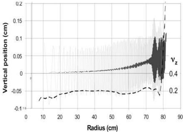
Figure 2: Vertical particle position as a function of radius when the coil is tilted 0.38 mrad. Dark line: particle starts at centre of iron gap, grey line: particle starts 1 mm above centre. Dashed line:  $\nu_z$ .
