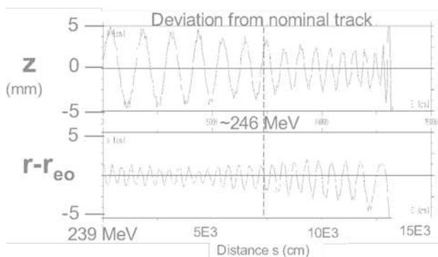
Figure 5: Track of an accelerated particle relative to the reference track starting at 239 MeV. The vertical deviation (top) and the horizontal deviation (bottom) are shown as a function of covered distance. The horizontal scale represents a distance covering  $\sim 30$  turns.
