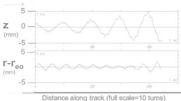
Figure 4: Track of a particle relative to the 246 MeV equilibrium orbit in the vertical plane (top) and in the horizontal plane (bottom).
