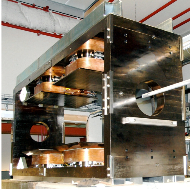
SR spin-rotator (and separator) magnet
